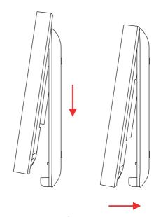
2. Attach the front panel onto the rear panel.
